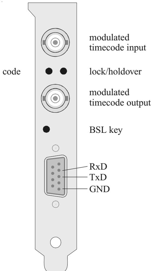
The bracket of the board includes the BNC-connectors for the amplitude modulated time codes (input/output), two LEDs, a key for activating the Bootstrap-Loader and a 9 pin D-Sub-plug.
