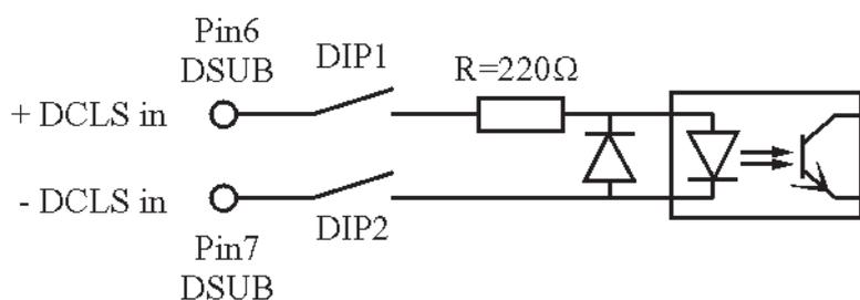
The internal series resistance allows direct connection of input signals with a maximum high level of +12 V (TTL or RS-422 for example). If signals with a higher amplitude are used, an additional external series resistance must be applied for not exceeding the limit of the forward current of the input diode (50 mA). The forward current should not be limited to a value of less than 10 mA to ensure save switching of the photocoupler.
